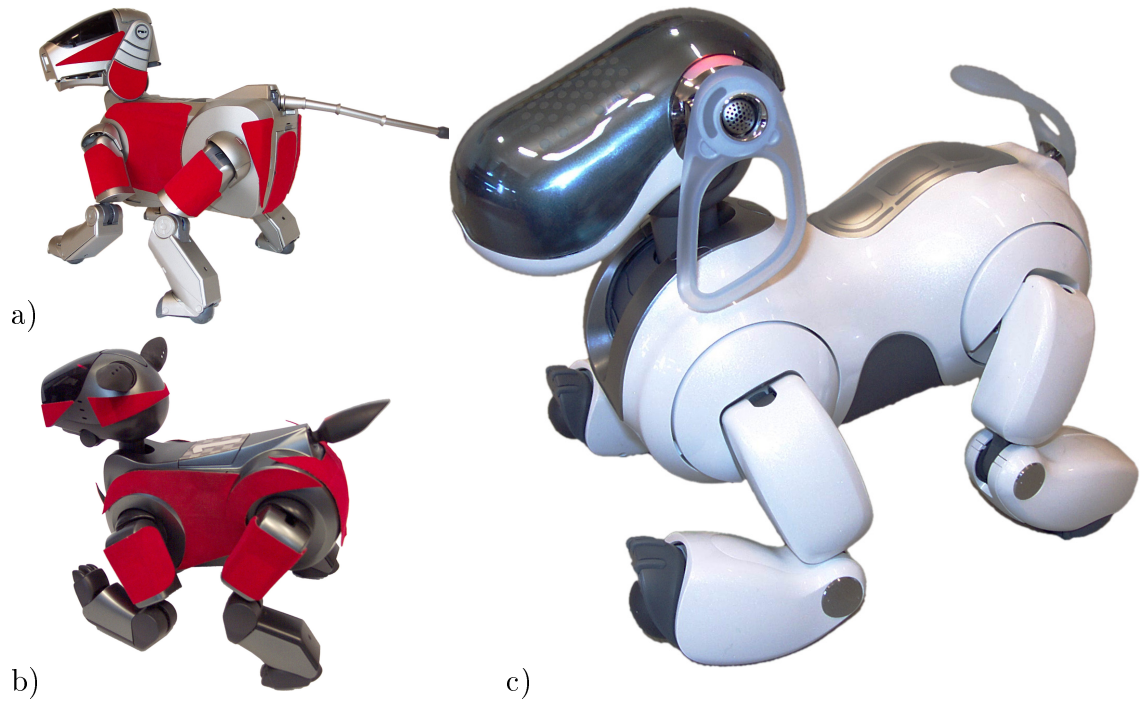
Figure 1.1: The robots used, partially with tricots, all in typical posture: a) ERS-110, b) ERS-210, c) ERS-7
